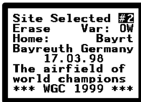
Before you load a new site into the SN10, you must erase the current site here. Place the cursor on **Erase** and press **ENTER** to erase the selected site.
