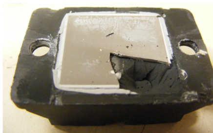
Image 6: bottom view ceramic substrate: substrate has cracked through centreline of ceramic. Resistor is open circuit. Heat damage on potting material located above resistor tile.
